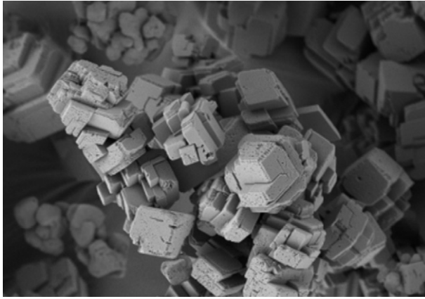
FIG. 55. SEM image of \text{CaCO}_3 particles obtained from water sample treated by pulsed nanosecond discharge [130].
