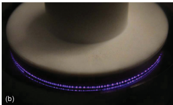
FIG. 8. Pulsed multichannel discharge array in water generated by two stainless steel disk electrodes separated by a dielectric layer [66].
